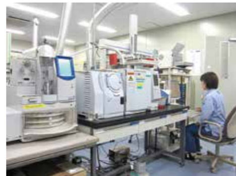
Organic substance examination using GC-MS
