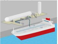
A vessel berths at a quay/pier where fuel can be supplied, and fuel is supplied from shore facilities to the ship.
