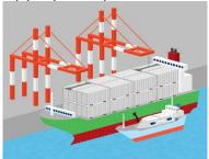
A bunkering vessel berths to a vessel arriving at/departing from a quay/pier, and fuel is supplied from the bunkering vessel to another vessel.
