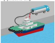
The vessel berths at the quay, and fuel is supplied by the lorry to the vessel.
